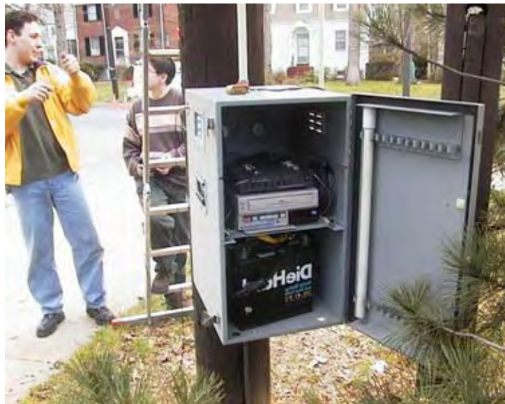
Figure 3. Portable Archival Traffic History (PATH) video system.
