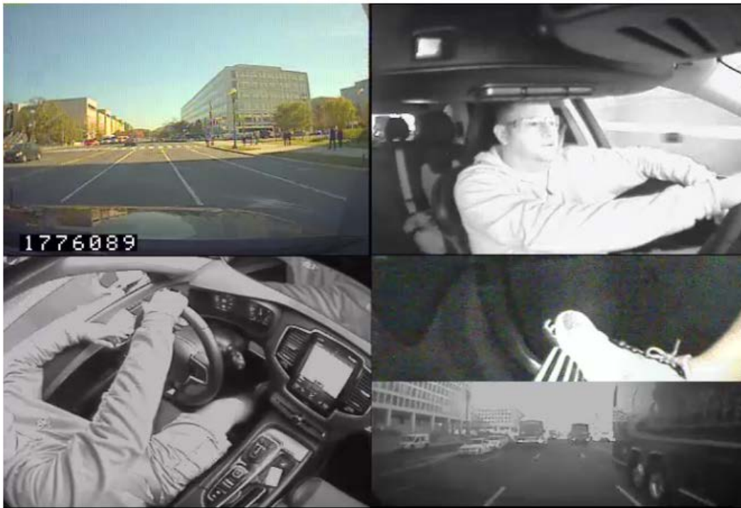
Figure 1. Data Acquisition System camera views
