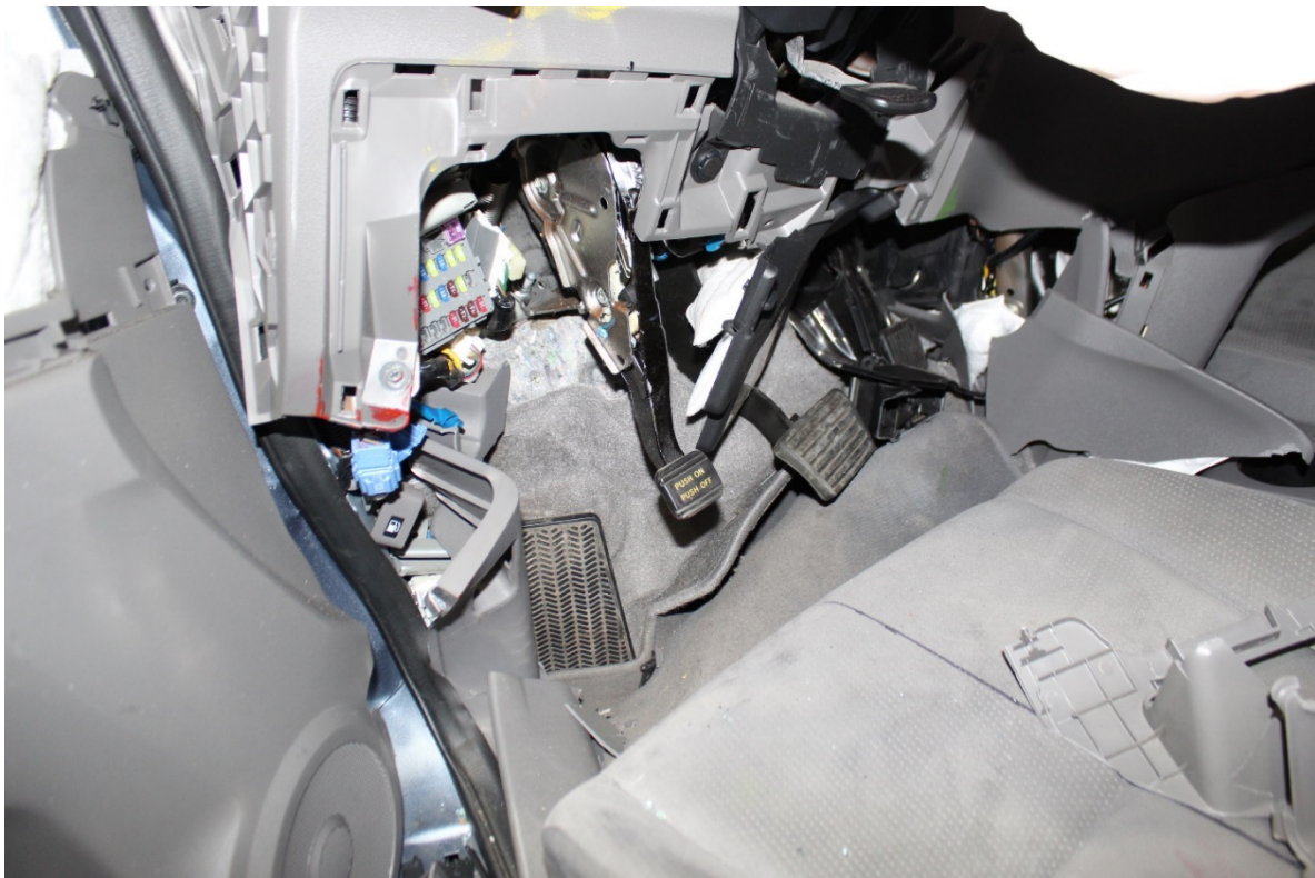
Significant footwell intrusion
