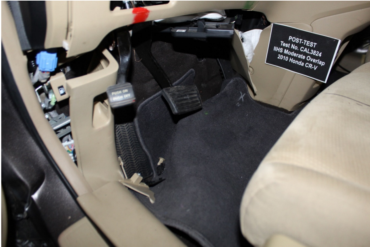
Footwell intrusion after displacing the dummy
