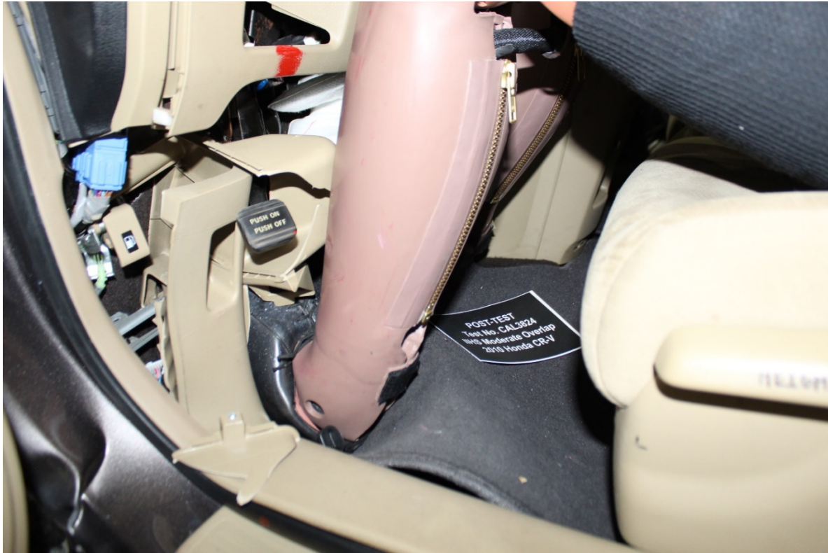
Left lower leg and footwell intrusion after the crash test
