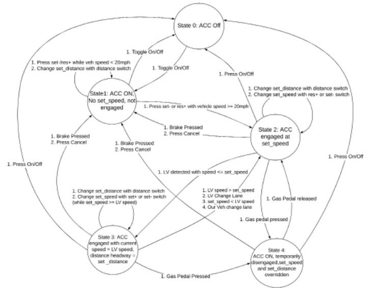
State Diagram for a Generic Adaptive Cruise Control System (LV = lead vehicle).
