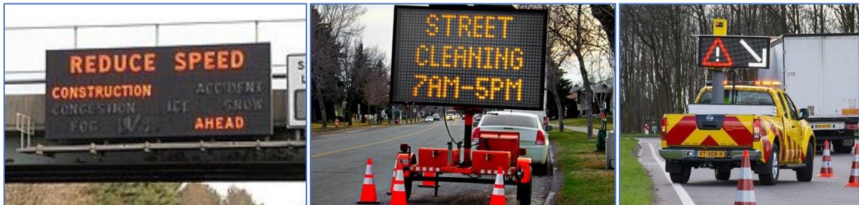
*Figure 3. Permanent VMS, portable VMS, and truck-mounted VMS.
