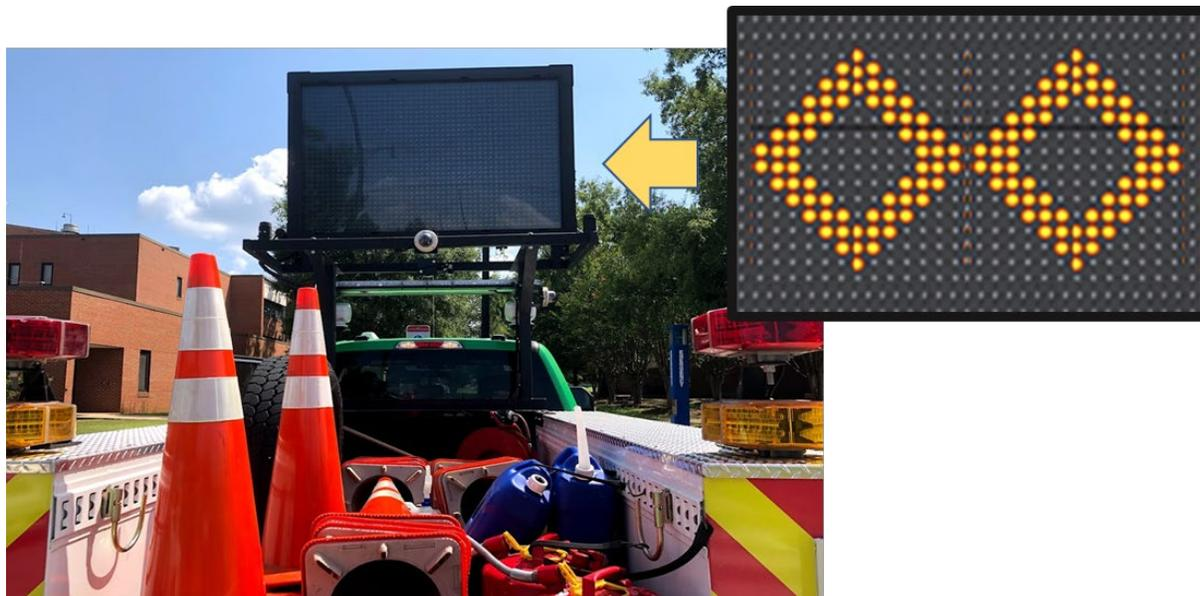
*Figure 6. Flashing diamond sign used as a default mode when the VMS board position is activated.*
