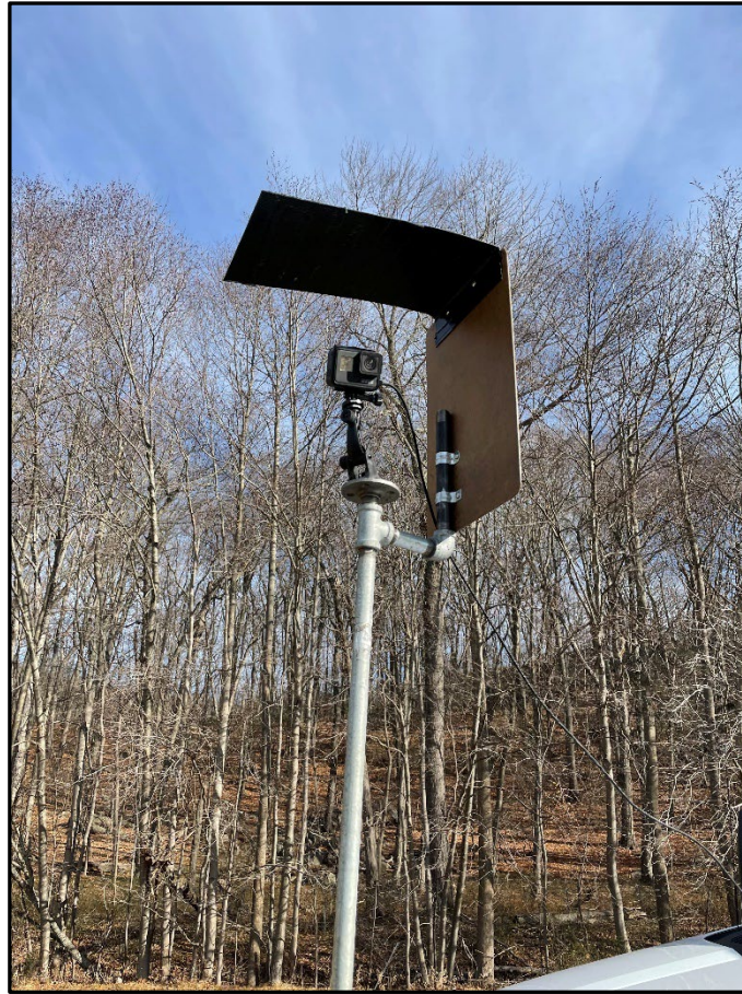
Figure 11. IR camera and light shade mounted on front bumper of wrecker.
