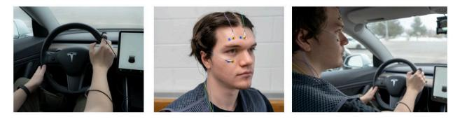
*Figure 3. The DRT vibrotactile stimulus and microswitch response button setup (left), EEG electrode setup (middle), and the combination of the two while driving (right).*
