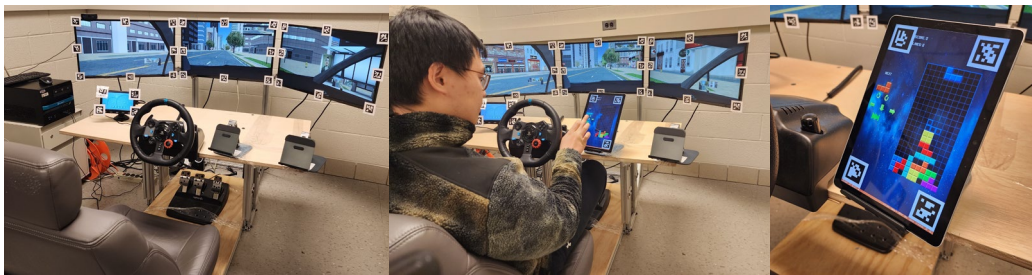
Figure 1. RTI driving simulator (left) and non-driving related task (Tetris) (center, right).
