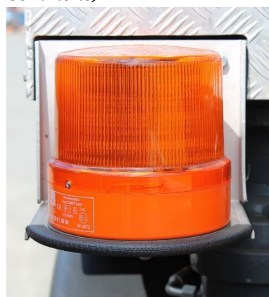
Figure 7. LED beacon (source: indeedous / Wikimedia Commons)
