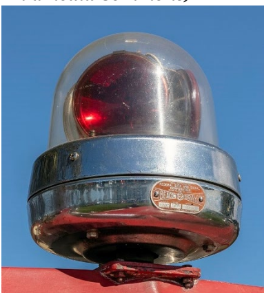
Figure 5. Rotating beacon (source: Acroterion / Wikimedia Commons)
