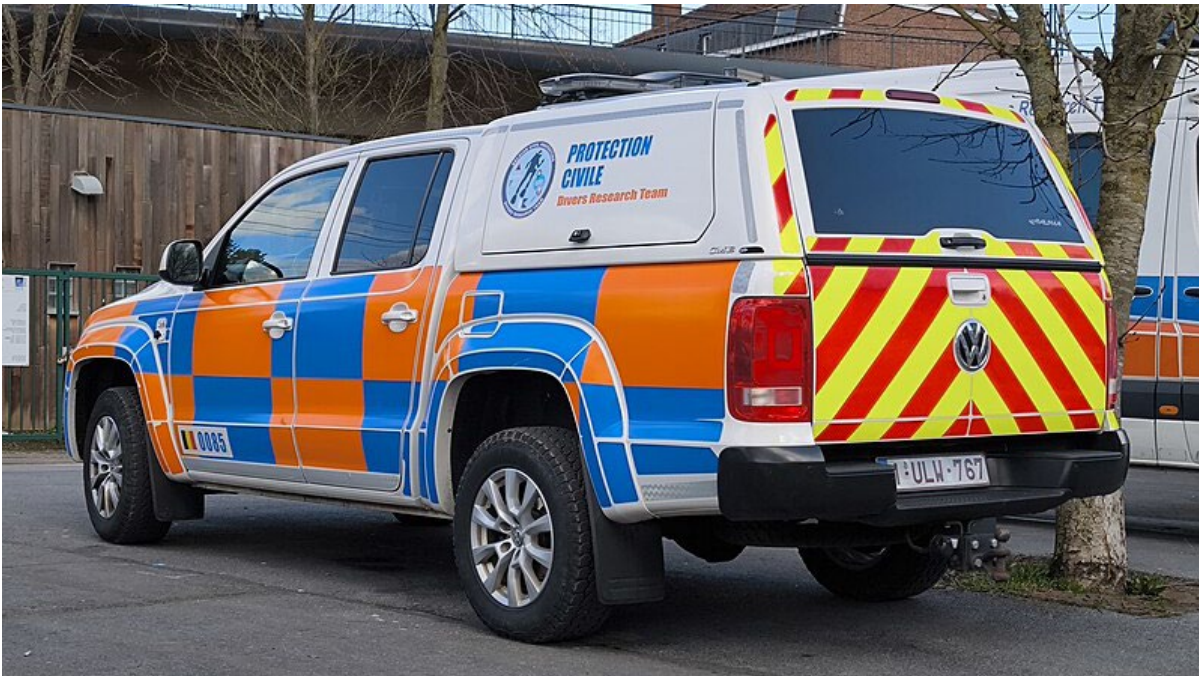
Figure 18. Checkerboard (Battenburg) markings (sides) and inverted-V markings (rear) of a Belgian Civil Protection vehicle (Source: Watopia2451/Wikimedia Commons (CC 3.0)).
