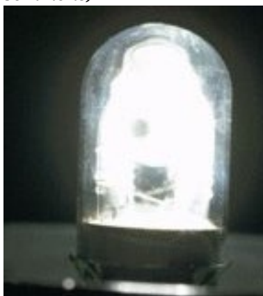
Figure 6. Xenon flash tube (source: C30/Wikimedia Commons)
