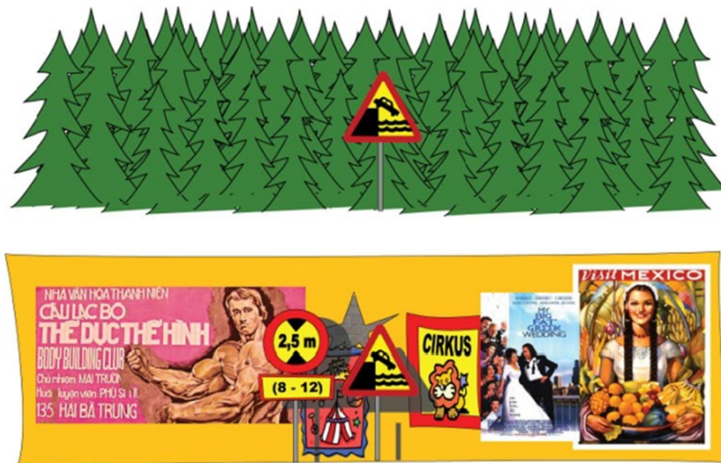
Figure 8. An object's conspicuity depends on the background environment (Source: Porathe and Strand, 2011).
