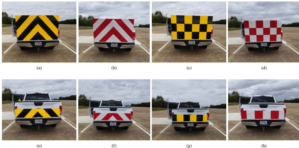
Figure 20. Marking combinations tested by Ullman et al. (2024)
