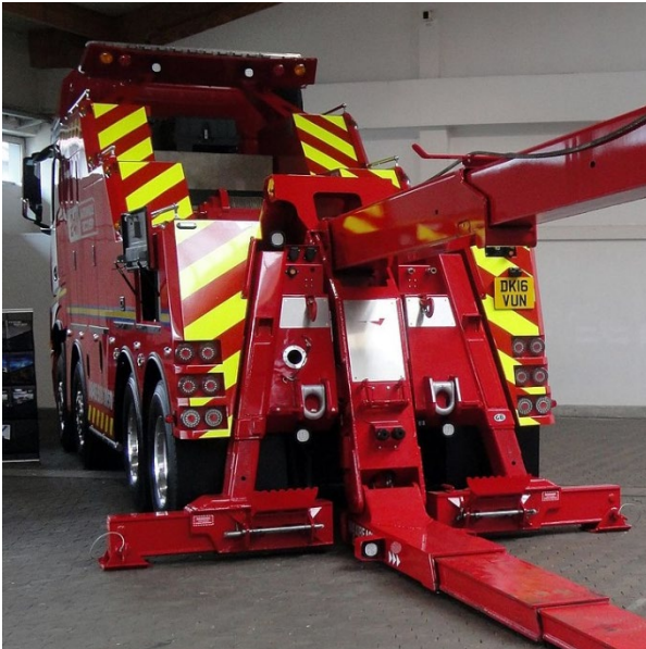
Figure 18. Checkerboard (Battenburg) markings (sides) and inverted-V markings (rear) of a Belgian Civil Protection vehicle (Source: Watopia2451/Wikimedia Commons (CC 3.0)).
