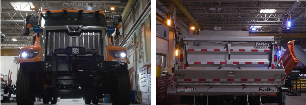
Figure 14. Minnesota DOT highway maintenance vehicle lighting (Source: MnDOT 2024).
