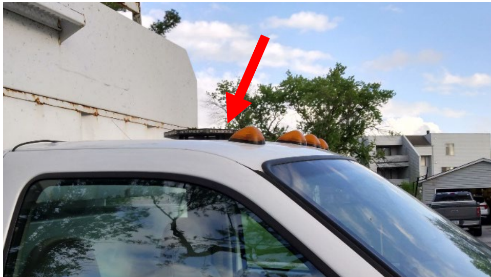
Figure 12. Low profile warning light on a work truck (Source: John Shaw/Safety Analytics International).
