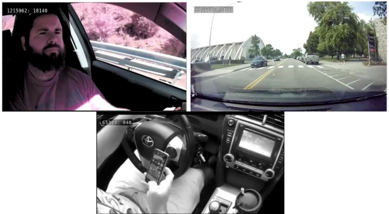
Figure 14. Camera views collected by VTTI MicroDAS (VTTI employee shown).
