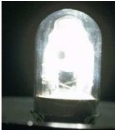
Figure 6. Xenon flash tube (source: C30/Wikimedia Commons)
