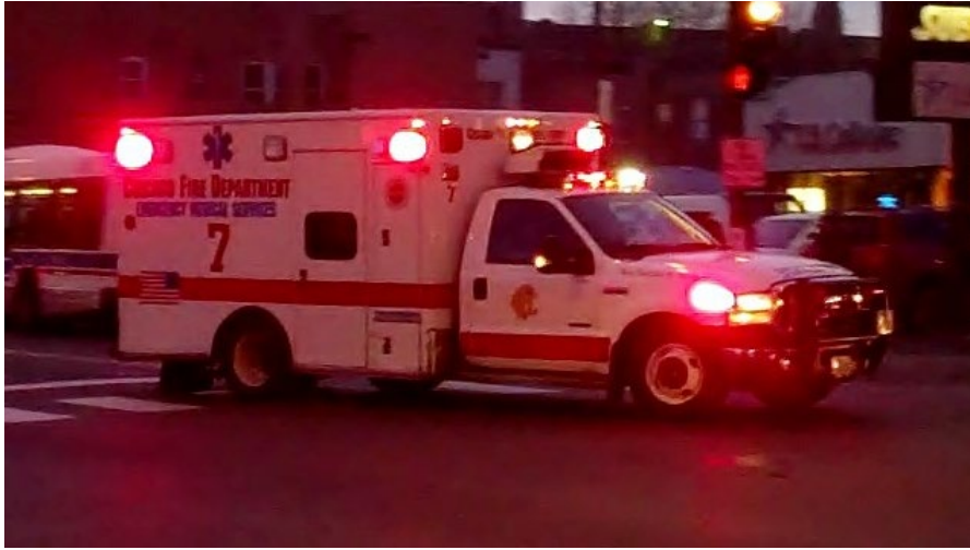
Figure 13. Ambulances based on the Federal “Star of Life” specification use several large lights mounted around the perimeter of the vehicle (Source: Arvell Dorsey, Jr./Wikimedia Commons (CC 2.0)).
