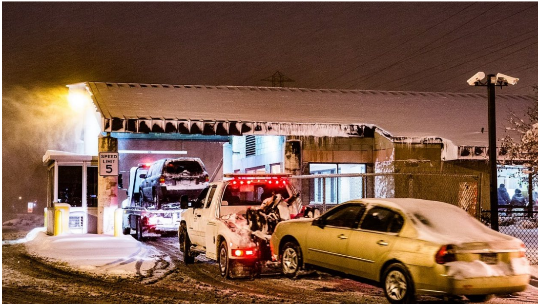
Figure 15. Loading equipment and the vehicle being towed/hailed often block the view of much of a tow truck's rear (Source: Tony Webster/Wikimedia Commons).
